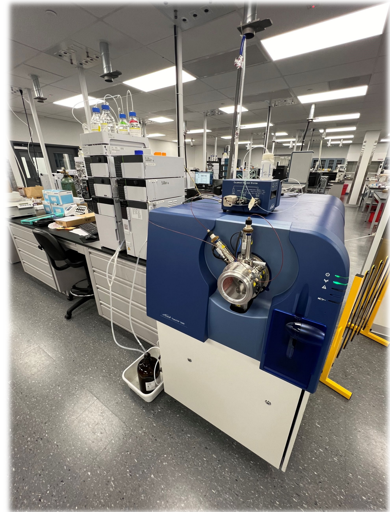
Sciex TripleTOF® 5600+ LC-QTOF coupled to a Shimadzu Nexera UHPLC
