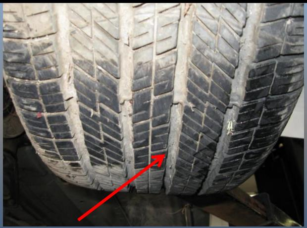
Underside of tire reveals tire damage due to sliding on asphalt.
